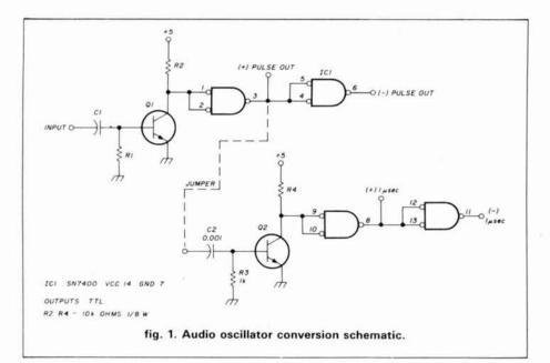
pulse with polarity selected from the IC1 outputs as shown.
